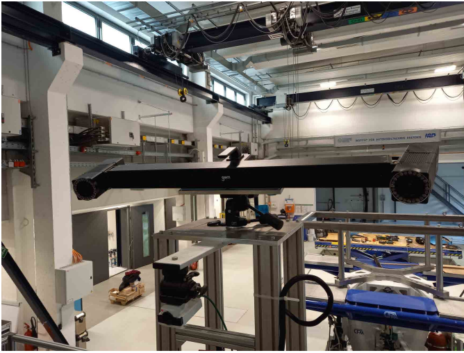
Figure 3. Setup of the “Aramis SRX optical measuring system” test stand [43].
