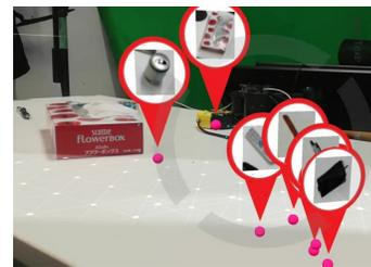
Fig. 3. Icons that display displaced objects in the AR application [5].
