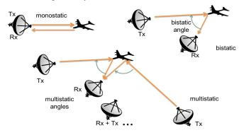
Figure 3. Monostatic, bistatic and multistatic radar systems.
