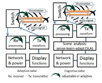
Figure 1. Simplified diagrams of adaptive and cognitive radars.
