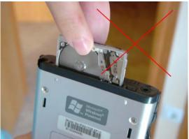
It is not recommend touching the plastic cover, especially in the place where the reading head is located. Never touch the cover when the Microdrive is running.
