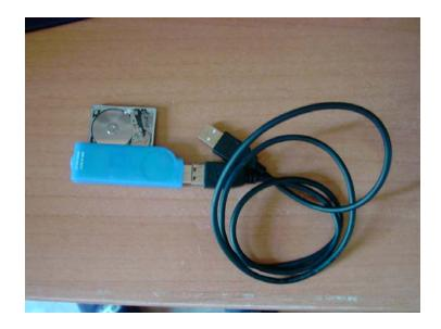
This very rare problem can be solved with a cable as the shown in the following picture, which takes the power from two USB connectors. Or you could buy a better quality extender USB cable.
