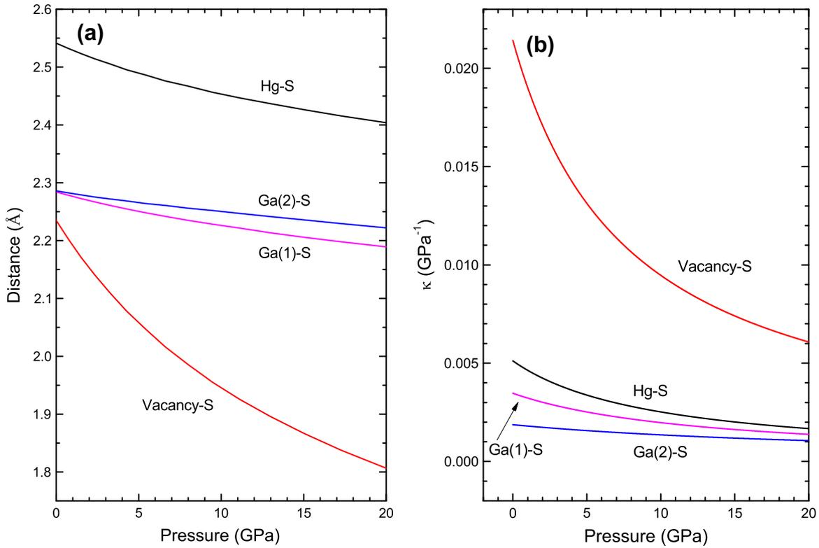
Fig. 6. (a) Calculated cation–anion and vacancy–anion distances, and (b) distance compressibilities as a function of pressure for DC-HgGa<sub>2</sub>S<sub>4</sub>.
