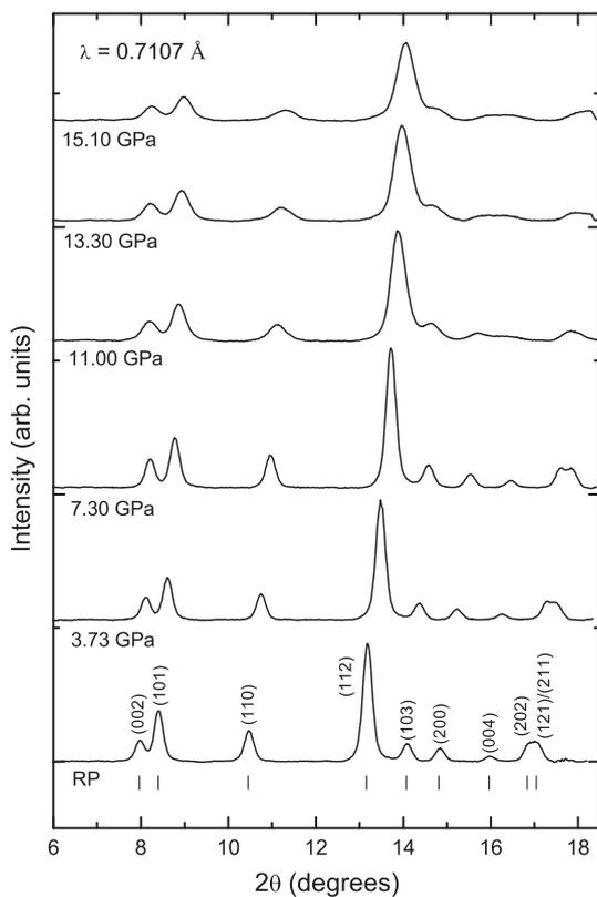
**Fig. 1.** Room temperature XRD patterns of HgGa<sub>2</sub>S<sub>4</sub> at different pressures from RP up to 15.1 GPa. In all diagrams, the background was subtracted. In the XRD pattern at RP, Bragg reflections are indicated with vertical ticks.
