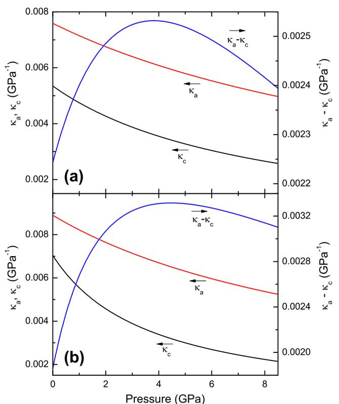
**Fig. 5.** Left side of panel:  $\kappa_a$  and  $\kappa_c$  vs. pressure. Right side of panel:  $(\kappa_a - \kappa_c)$  vs. pressure. Results correspond to: (a) XRD experiments, and (b) PBEsol calculations.
