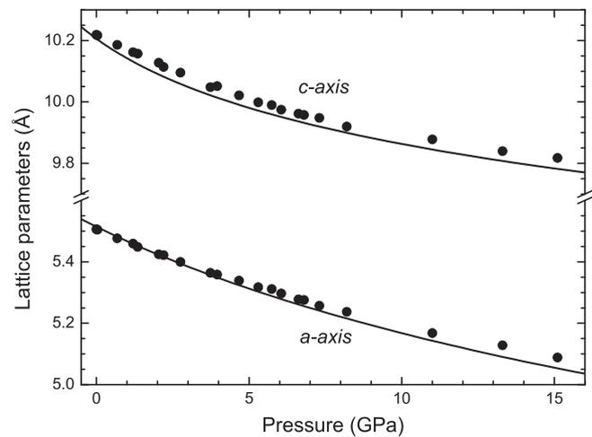
**Fig. 2.** Lattice parameters of the DC phase of HgGa<sub>2</sub>S<sub>4</sub> as a function of pressure. Symbols refer to experimental data. Theoretical results are plotted with solid line.
