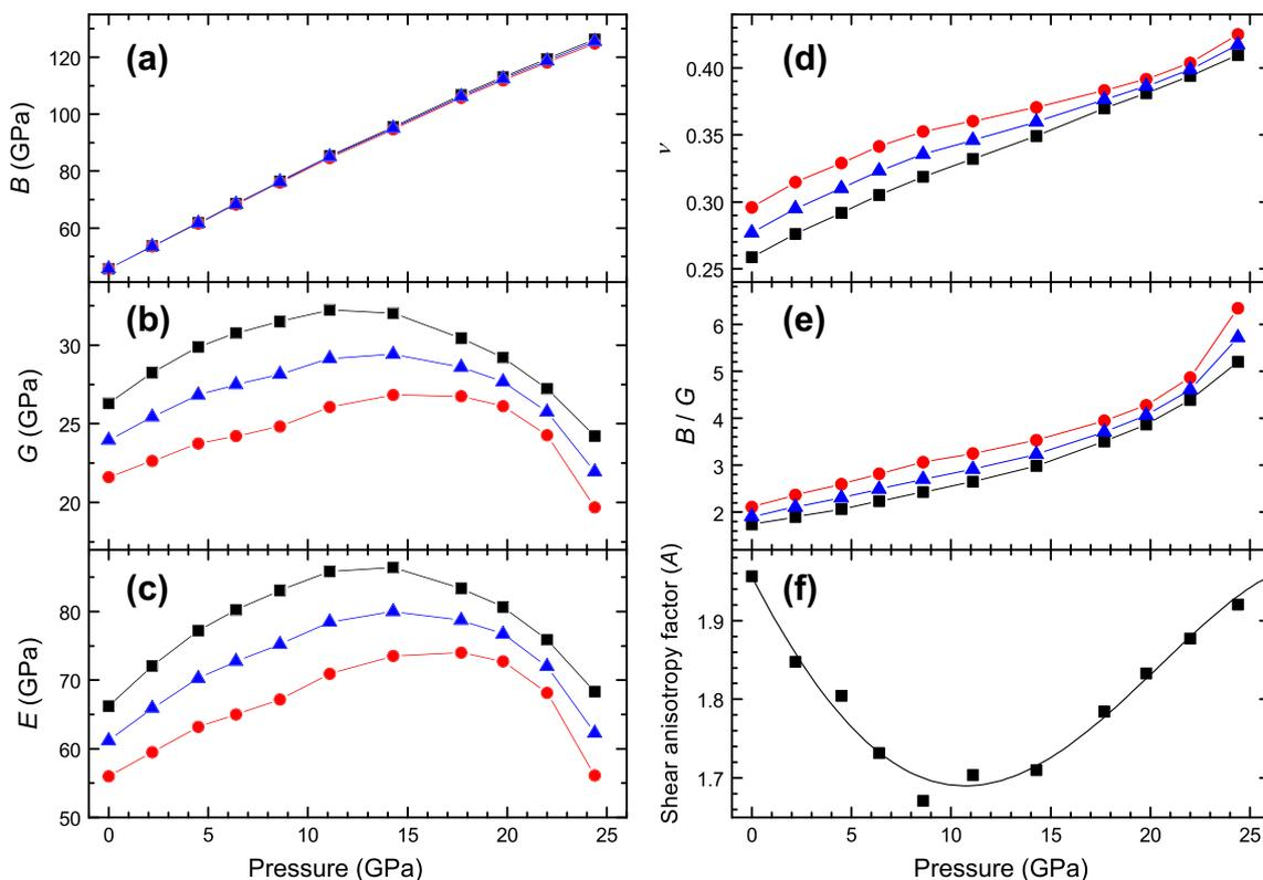
**Fig. 8.** Pressure dependence of (a)  $B$ , (b)  $G$ , (c)  $E$ , (d)  $\nu$ , (e)  $B/G$ , and (f)  $A$ . Squares, circles, and triangles refer to the Voigt, Reuss, and Hill approximations; respectively. Data for the  $A$  anisotropy factor are shown for  $\phi_\kappa = 3.72^\circ$ . Solid lines connecting the calculated data points are guides to the eyes in panels (a) to (e). Solid line in panel (f) represents the behavior of  $A$  with pressure.
