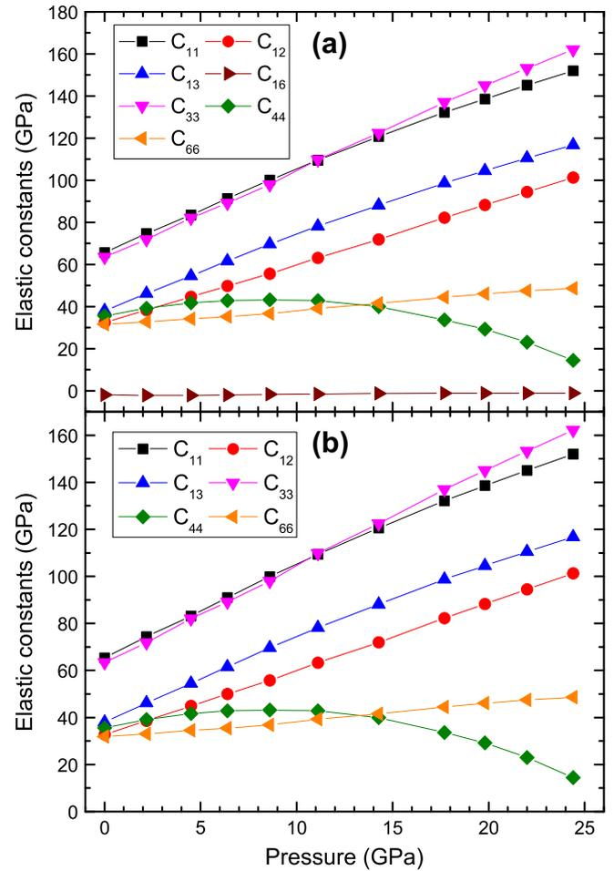
Fig. 7. Pressure dependence of the theoretical elastic constants of DC- $\text{HgGa}_2\text{S}_4$ : (a) Seven  $C_{ij}$  elastic constants and (b) Six  $C_{ij}$  elastic constants. The calculated data points are guides to the eyes.
