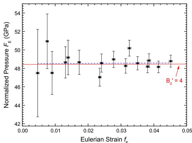
**Fig. 4.** Volume–pressure data of DC- $\text{HgGa}_2\text{S}_4$  displayed as a plot of the normalized pressure  $F_E$  against the Eulerian strain  $f_E$ . The blue dashed line is a linear fit to experimental  $F_E$ – $f_E$  data. Solid red line represents the case of a BM2 EOS with  $B'_0 = 4$ . (For interpretation of the references to color in this figure legend, the reader is referred to the web version of this article.)
