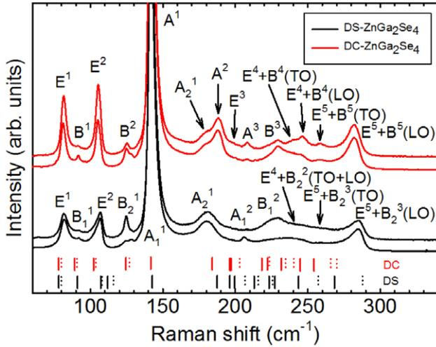
**Figure 3.** Unpolarized RT Raman spectra of DS-ZnGa<sub>2</sub>Se<sub>4</sub> (black, bottom) and DC-ZnGa<sub>2</sub>Se<sub>4</sub> (red, top) in two different parts of the samples. Labels refer to symmetry assignments for the Raman modes in the DS and DC structures. *Ab initio*-calculated values of the TO (solid) and LO (dotted) first-order Raman-active mode frequencies for both DS (DC) samples are marked with vertical black (red) marks at the bottom.
