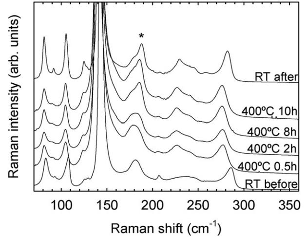
**Figure 2.** Unpolarized Raman spectra of ZnGa<sub>2</sub>Se<sub>4</sub> before, during and after thermal annealing at 400 °C. The asterisk marks the strong new mode that appears after heating the DS sample at 400 °C for 10 h. This mode ( $A^2$ ) is characteristic of the DC phase and it is absent from the DS phase. Note that the equivalent mode in the DS phase is the  $A_2$  mode, which is silent but can be observed by defect-assisted Raman scattering (see text).
