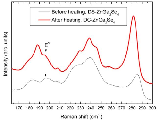
**Figure 4.** Polarized RT Raman spectra taken in backscattering geometry along the (111) direction with crossed polarization in a direction close to [110] for as-grown DS- $\text{ZnGa}_2\text{Se}_4$  (black, bottom), and after heating at 400  $^\circ\text{C}$  for 10 h resulting in DC- $\text{ZnGa}_2\text{Se}_4$  (red, top). The cooling rate was always 1  $^\circ\text{C min}^{-1}$ .
