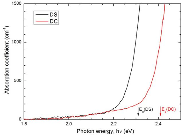
**Figure 5.** RT optical absorption spectra of DS- $ZnGa_2Se_4$  (black) and DC- $ZnGa_2Se_4$  (red) samples. Arrows indicate the experimental direct bandgap energies in both phases.
