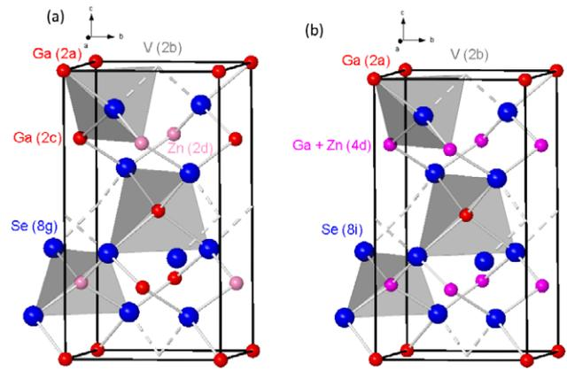
**Figure 1.** Scheme of atoms in  $\text{ZnGa}_2\text{Se}_4$  in DC structure (a) and DS (model 2 in [27]) structure (b). Large (blue) atoms are Se, small dark (red) atoms are Ga, and small light (magenta) atoms are Zn. Mixed Ga and Zn atoms in DS structures are shown in rose color. For the sake of clarity Wyckoff sites are given in parenthesis.
