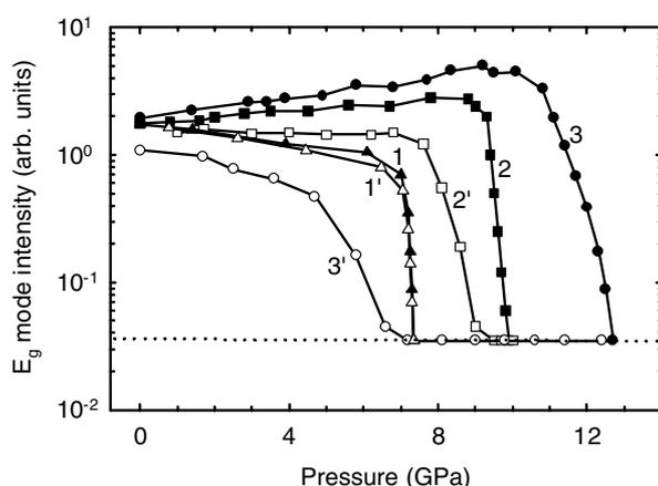
**Figure 5.** The pressure dependence of the intensity of the  $E_g$  mode in  $MnIn_2S_4$  (curve 1, triangles),  $CdIn_2S_4$  (curve 2, squares), and  $MgIn_2S_4$  (curve 3, circles). Full symbols correspond to upstroke runs and open symbols to downstroke runs. The horizontal line indicates the sensitivity level of the experimental set-up.
