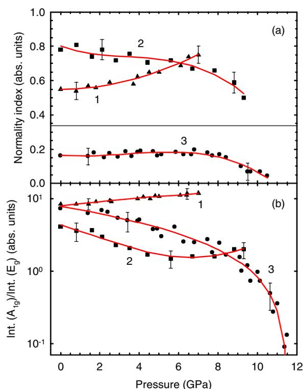
**Figure 6.** Pressure dependences of the normality index (a) and of the integral intensity of the  $A_{1g}$  mode normalized to the intensity of  $E_g$  mode (b) for  $\text{MnIn}_2\text{S}_4$  (curve 1, triangles),  $\text{CdIn}_2\text{S}_4$  (curve 2, squares), and  $\text{MgIn}_2\text{S}_4$  (curve 3, circles). The curves are guides for the eye.
