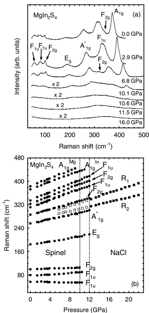
**Figure 3.** (a) Raman spectra of  $\text{MgIn}_2\text{S}_4$  at various pressures. (b) Raman shifts as a function of pressure in  $\text{MgIn}_2\text{S}_4$ . The vertical dashed lines delimit the region where the  $\text{LiVO}_2$ -type NaCl superstructure is observed. Error bars are not indicated for the sake of clarity.
