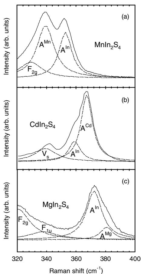
**Figure 4.** Spectral decomposition of the Raman spectra of  $\text{MnIn}_2\text{S}_4$  (a),  $\text{CdIn}_2\text{S}_4$  (b), and  $\text{MgIn}_2\text{S}_4$  (c) at zero pressure in the vicinity of  $A_{1g}(\text{M}^{\text{II}})$  and  $A_{1g}(\text{In}^{\text{III}})$  modes.
