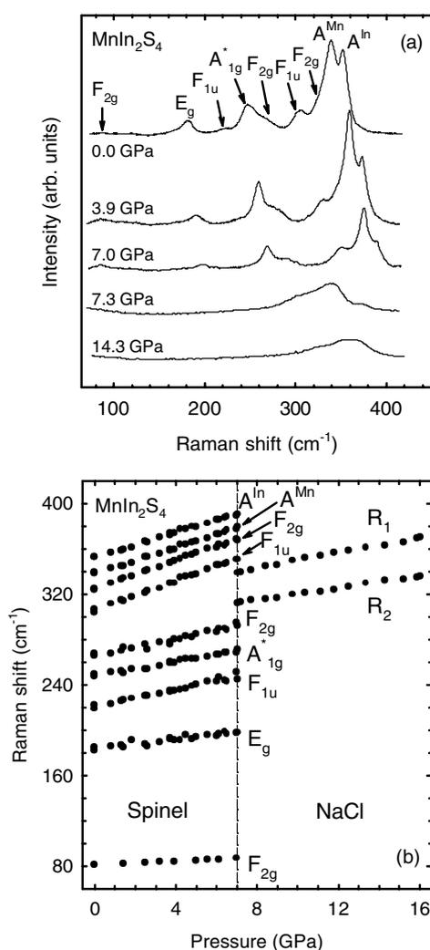
**Figure 1.** (a) Raman spectra of  $\text{MnIn}_2\text{S}_4$  at various pressures. (b) Raman shifts as a function of pressure in  $\text{MnIn}_2\text{S}_4$ . The vertical dashed line indicates the pressure at which the phase transition between the spinel and the NaCl structures occurs. Error bars are not indicated for the sake of clarity.
