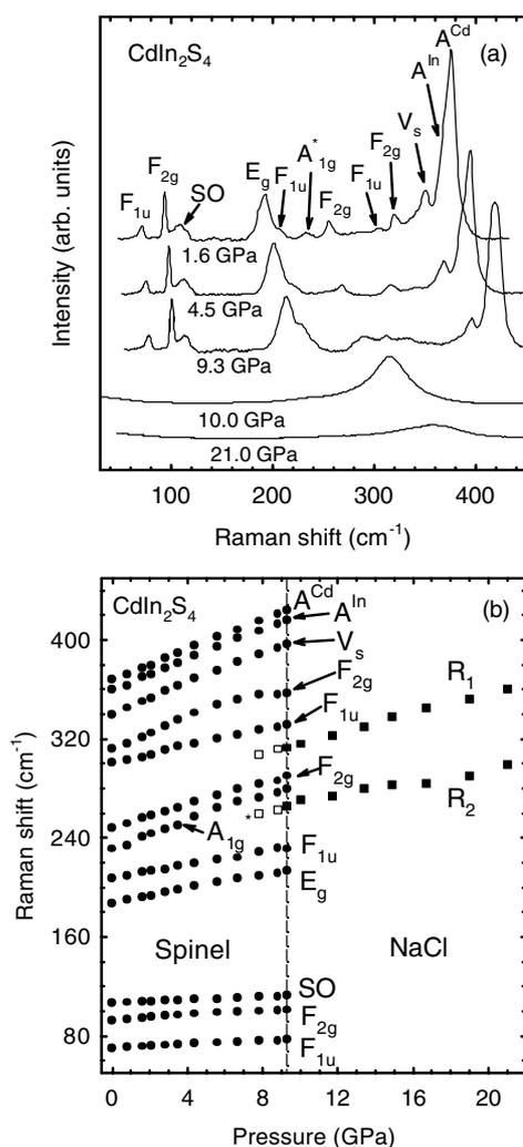
**Figure 2.** (a) Raman spectra of  $\text{CdIn}_2\text{S}_4$  at various pressures. (b) Raman shifts as a function of pressure in  $\text{CdIn}_2\text{S}_4$ . The vertical dashed line indicates the pressure at which the phase transition between the spinel and the NaCl structures occurs. Error bars are not indicated for the sake of clarity.
