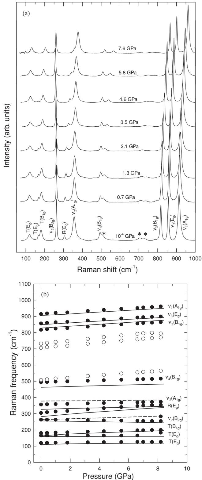
FIG. 1. (a) Raman spectra of  $\text{ScVO}_4$  in the zircon phase between 1 atm and 7.6 GPa. Asterisks represent the second-order Raman modes. (b) Pressure dependence of the Raman mode frequencies in zircon-type  $\text{ScVO}_4$  (solid symbols). Empty symbols are likely second-order Raman modes. The solid lines are the calculated modes. The dashed lines represent Raman modes not observed in the experiments.
