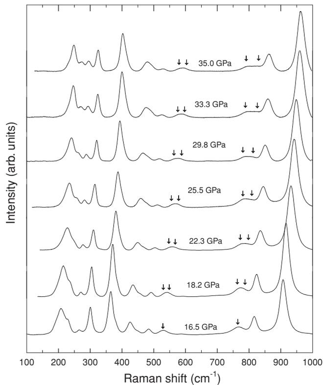
FIG. 3. Raman spectra of the HP fergusonite phase of  $\text{ScVO}_4$  between 18.2 and 35 GPa. The Raman spectrum of the scheelite phase at 16.5 GPa is also shown for comparison. Arrows show the two modes that exhibit considerable broadening upon compression.
