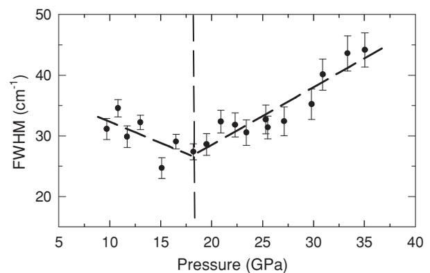
FIG. 4. FWHM of the mode assigned as  $\nu_3(E_g)$  in the scheelite phase between 9.7 and 35 GPa. The broadening beyond 18.2 GPa evidences the phase transition.
