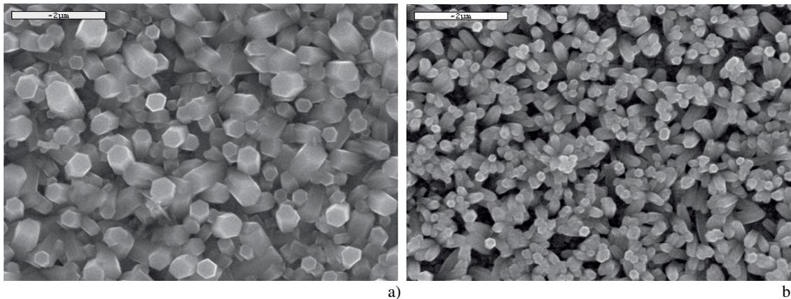
**Fig. 1** SEM micrographs of ZnO nanocolumns grown under different conditions: (a) ZED1 sample:  $I = 2.5 \text{ mA/cm}^2$ ;  $t = 30 \text{ min}$ ;  $T = 65 \text{ }^\circ\text{C}$ ; (b) ZED2 sample:  $I = 2.5 \text{ mA/cm}^2$ ;  $t = 10 \text{ min}$ ;  $T = 85 \text{ }^\circ\text{C}$ .
