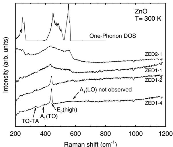
**Fig. 3** Room-temperature Raman spectra of nanocolumnar ZnO crystals as a function of the column size and annealing temperature. ZED1-1 and ZED2-1 correspond to as-grown crystals, ZED1-2 and ZED1-4 correspond to the ZED1 sample after annealing at 200 and 400 °C, respectively. The calculated one-phonon density of states from first principles in Ref. [7] is also shown for comparison.
