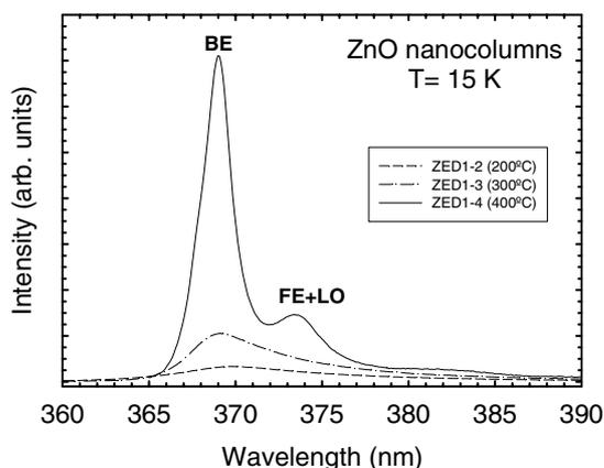
**Fig. 2** Low-temperature photoluminescence spectra of nanocolumnar ZnO crystals after annealing at different temperatures.
