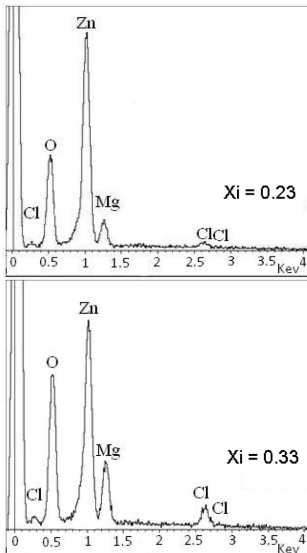
**Figure 1** EDS spectra of ZMO sprayed films at 300 °C with different Mg molar fraction in starting solution.
