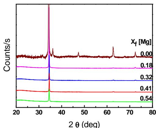
**Figure 3** XRD spectra of ZMO thin films with different Mg molar fraction.
