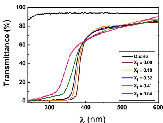
**Figure 6** Optical transmittance spectra of  $Zn_{1-x}Mg_xO$  thin films with different Mg molar fractions.
