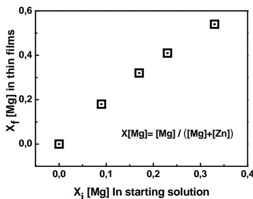
**Figure 2** Mg molar fraction ( $X_f$ ) in the ZMO thin films as a function of the Mg molar fraction in the starting solution ( $X_i$ ).
