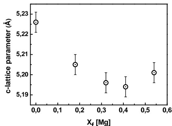
**Figure 4** Dependence of the c lattice parameter as a function of the Mg molar fraction in the ZMO thin films.
