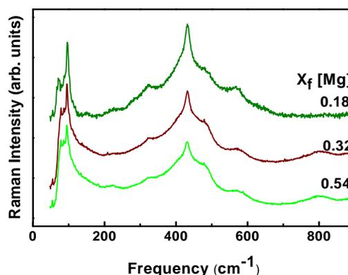
**Figure 5** Raman scattering measurements of ZMO thin films with different Mg molar fraction.
