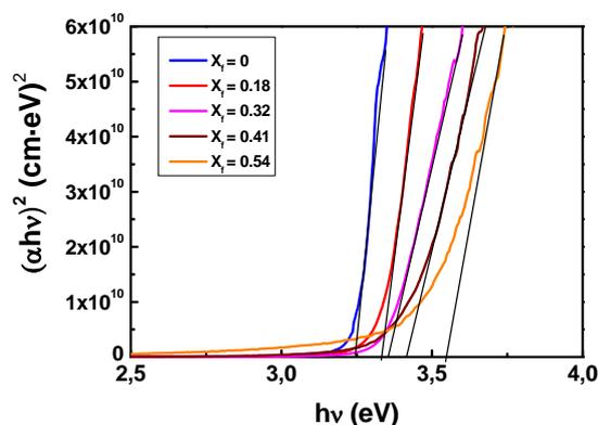
**Figure 7**  $(\alpha hv)^2$  vs. photon energy for  $Zn_{1-x}Mg_xO$  sprayed thin films with different Mg molar fraction.
