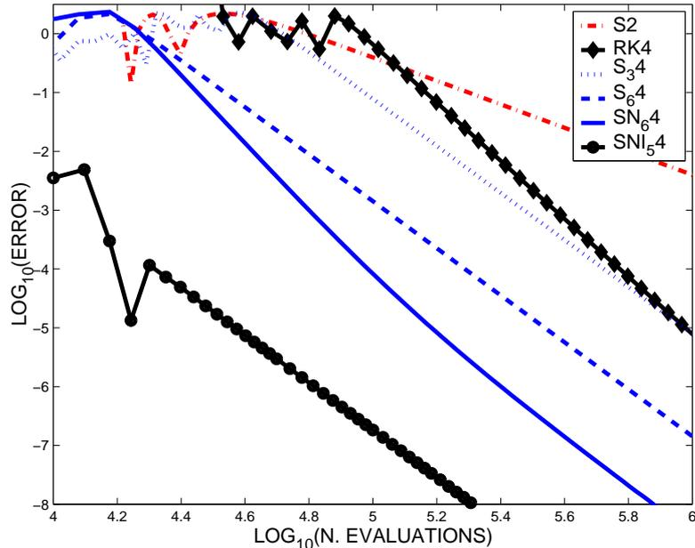
**Fig. 1.** Error in the solution  $(q_1(t_f), q_2(t_f))$  vs. the number of evaluations for different 4th-order splitting methods (the extra cost in the method SNI<sub>5</sub>4, designed for perturbed problems, is not taken into account).
