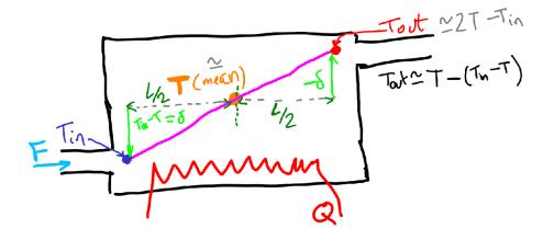
if the "mean" temperature is  $T=0.5T_{in}+0.5T_{out}$ , solving for  $T_{out}$  we get:  $T_{out}=2T-T_{in}$
