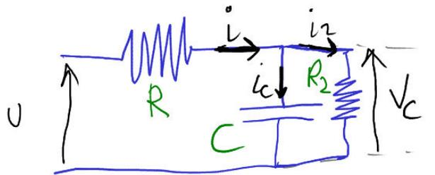
$$\frac{dV_c}{dt} = \frac{1}{C} i_c, \quad i_c = i - i_2, \quad i = \frac{1}{R} \cdot (u - V_c), \quad i_2 = \frac{V_c}{R_2}$$
