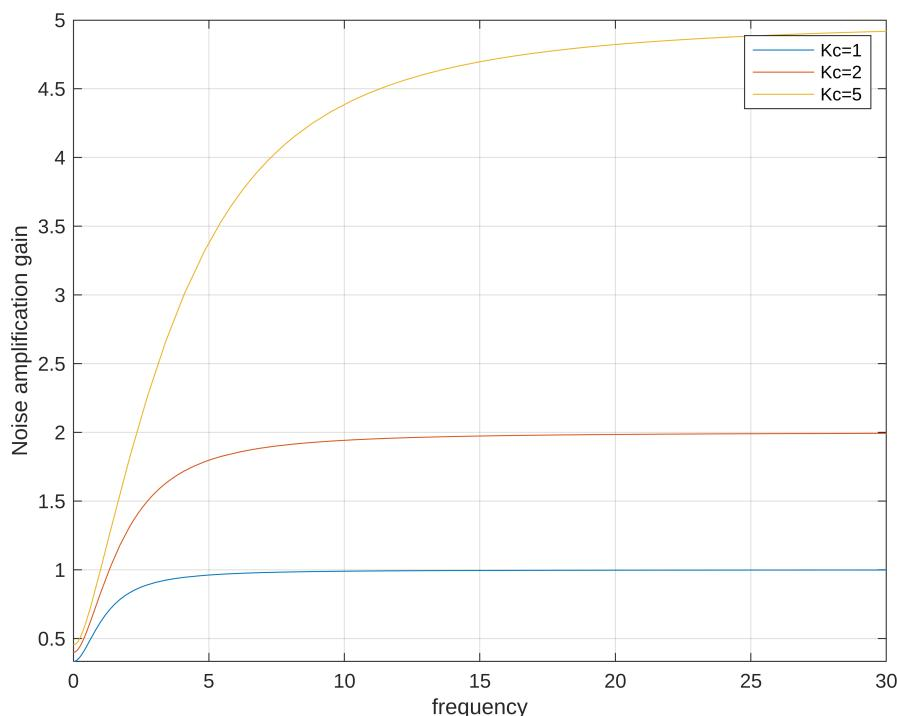
**Remark:** this is a NON logarithmic plot; usually you will see the "Bode" diagram, which has logarithmic scales both in "frequency" and "amplitude gain" axes.
