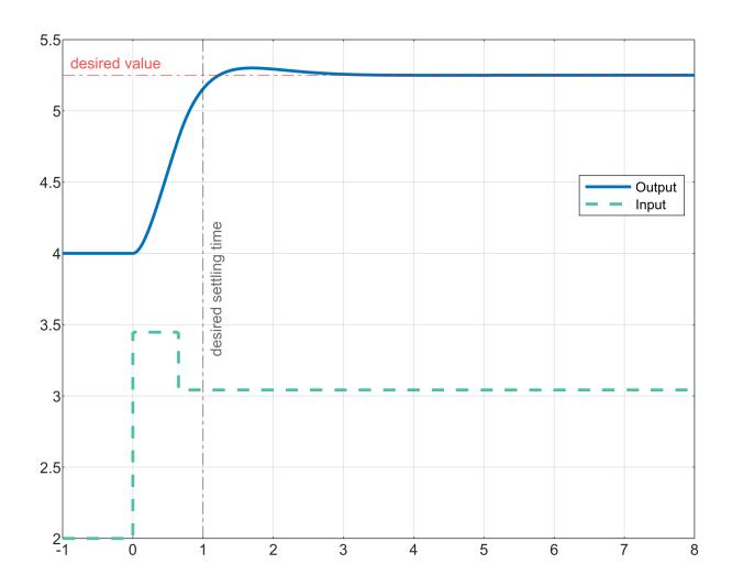
That is, we have designed a two-step input profile: an initial "boost" to climb up faster and then a "final" steady-state value to stay at the desired point. This is a "precomputed" input profile (open-loop control): no measurement is taken while the step sequence is being applied in order to decide when to switch.
