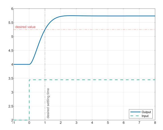
In order to avoid exceeding the desired final value, it will be necessary to switch to the input value that maintains the desired value in equilibrium once it is reached:
