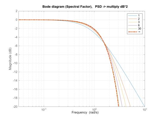
This is the actual amplitude correction so the integral of the "power spectral density" (i.e., variance) keeps constant to one:
