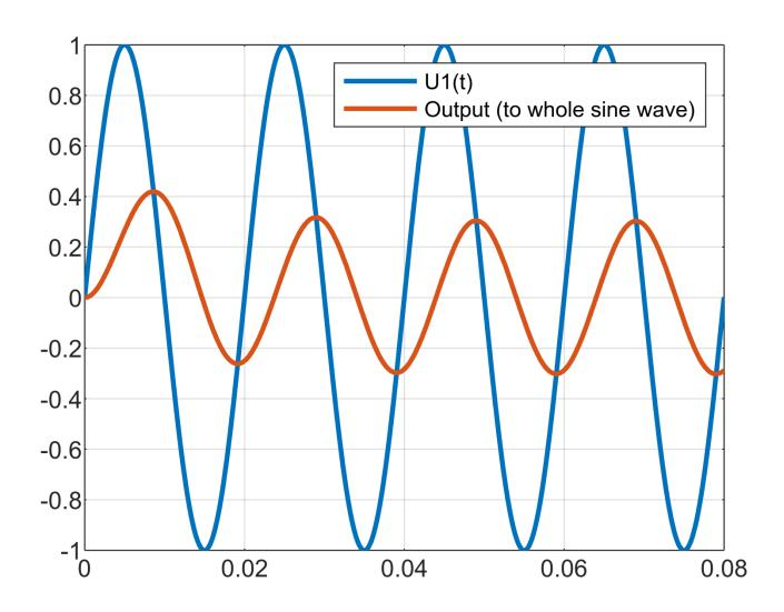
As we have a change in the input "formula" at t = 0.01, switching to "zero", the above solution is only valid in the first 0.01 seconds, being meaningless from that time onwards. For  $t \ge 0.01$  we will have a "free" response (zero input) from the initial conditions that the first semi-period have left the system at:
