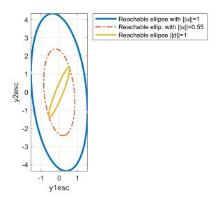
Indeed, we can see that the effect of u is larger than that of d, so u has no problems to counteract the "yellow" ellipsoid producing an output contrary to it inside the "red" ellipsoid.
