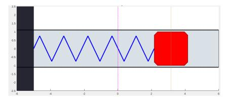
Let us solve the equation of a mass-spring-damper system (linearized, zero equilibrium; linear viscous friction assumed), starting at initial conditions out of equilibrium, written as:
