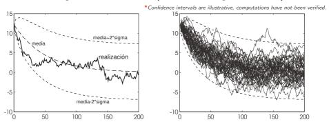
Mean, variance (or standard dev.) depend on time. They can be computed by "repetition of the experiment" (sample mean, etc.), *data-based* approach, or by *integration* of the differential equations of an RC circuit (in its *stochastic* version).
