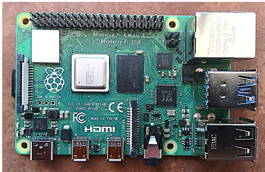
Figura 1.2. Raspberry Pi 4b, 2019, cara de componentes
