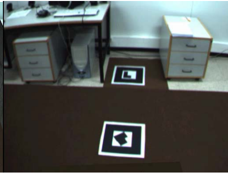
Fig. 6. Two of the three markers of the AR system
