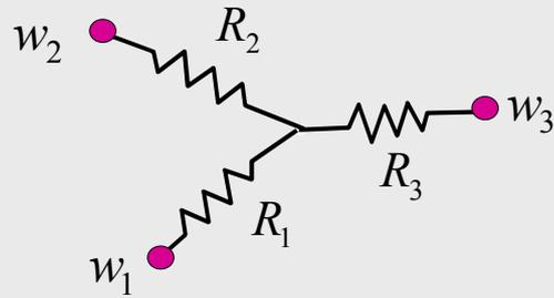
$$R_{12} = R_1 R_2 \left( \frac{1}{R_1} + \frac{1}{R_2} + \frac{1}{R_3} \right)$$
