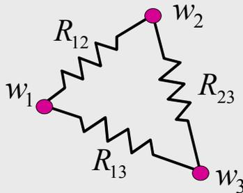
$$R_1 = \frac{R_{12} R_{13}}{R_{12} + R_{13} + R_{23}}$$
